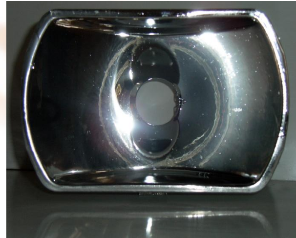
Headlight with reflector coating restored by ion-plasma method
